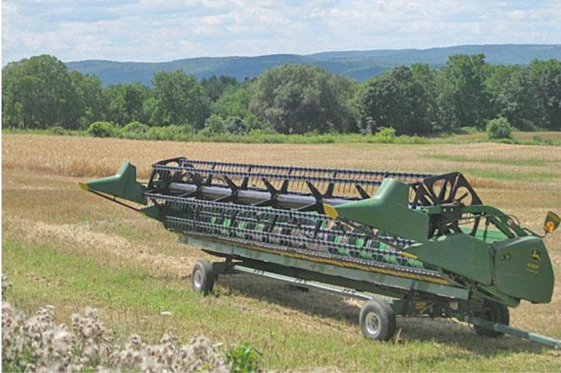
A small-grain header that attaches to a combine. *(Photo provided)*
