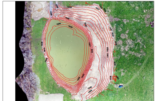
Richmyer Retention Pond "As-Built" Contour Map 1' Contour 1 inch = 67 feet
